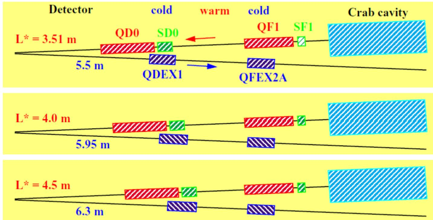
Figure 1: Magnets near IP for  $L^* = 3.51, 4.0, 4.5$  m.
