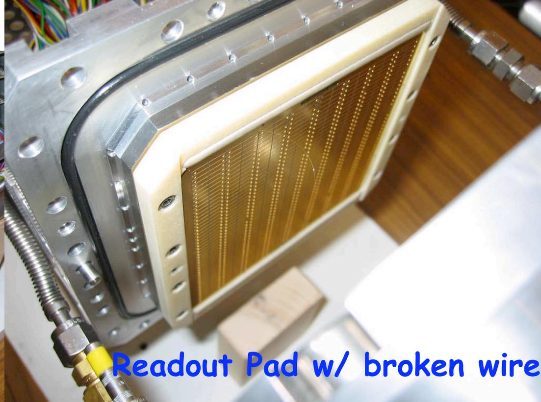
Readout Pad w/ broken wire
