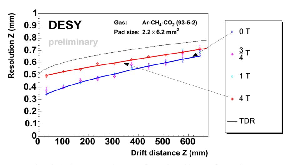
At very low drift distance: pad size too large for efficient charge sharing: reduced resolution
