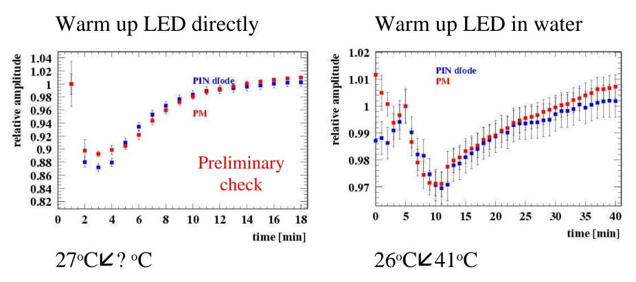
Consistent response of PM and PIN diode Direct warm up is too fast and T cannot be controlled
