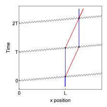
at x=0 on the left and emits pulse that propagate to the right at times 0, T, and 2T to implement the  $\frac{\pi}{2} - \pi - \frac{\pi}{2}$  sequence. The paths of the light pulses are shown in gray. The resulting atom paths are shown for both the ground (blue) and excited (red) states. Assume the excited state has energy  $\hbar\omega_A$  with respect to the ground state. The following trigonometric identities are useful for part 4:
