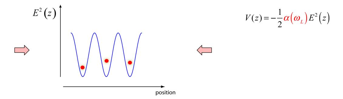
Optical lattice : counter-propagating laser beams = standing wave
