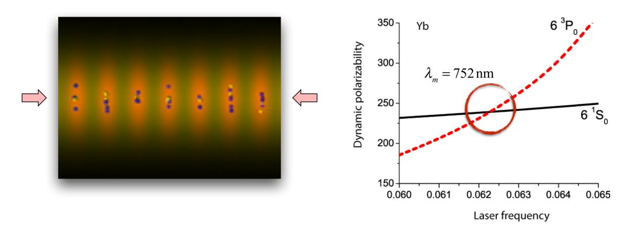
Tune laser frequency :: magic frequency (Katori)  $\alpha_{g}(\omega_{\text{magic}}) \equiv \alpha_{e}(\omega_{\text{magic}}) \implies \delta v_{\text{clock}} = 0$
