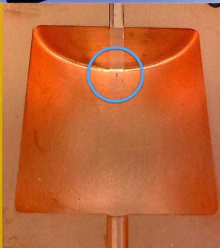
The electric field of individual photons exercises the nonlinear inductance of the Josephson junction. **Photon number is transduced into frequency shifts of the  $|g\rangle \rightarrow |e\rangle$  transition.** Same as Lamb shift, but for finite photon number.
