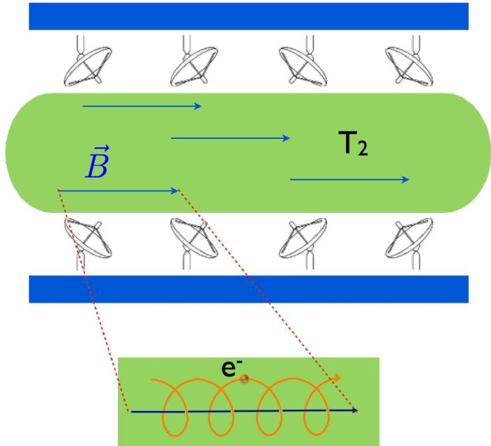
$$\omega(\gamma) = \frac{\omega_0}{\gamma} = \frac{eB}{E + m_e}$$
