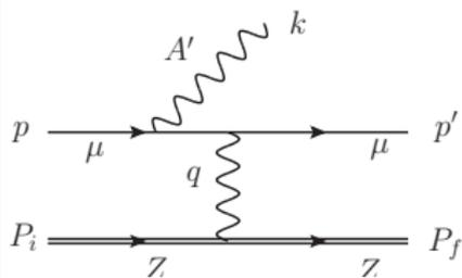
Brems. from initial muon state
