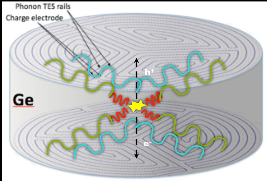
Charge electrodes: biased at +/- 2V, measure  $E_{recoil}$ , configured to reject surface events
