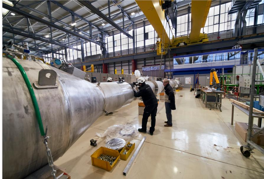
On Friday, 24 November, ARIA's top and bottom modules plus one standard module were brought to Building 180 and lined up to precisely test their alignment and interconnections. (Image: Max Brice/CERN)
