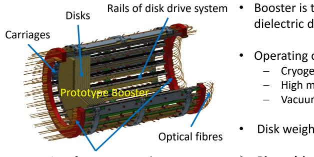
Laser interferometer couplers
