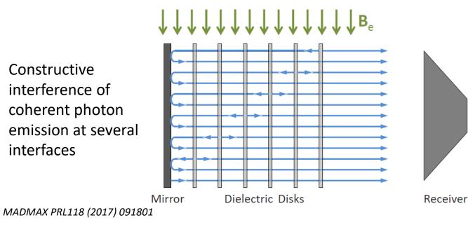
Output power P of the dielectric haloscope per unit area A is:
