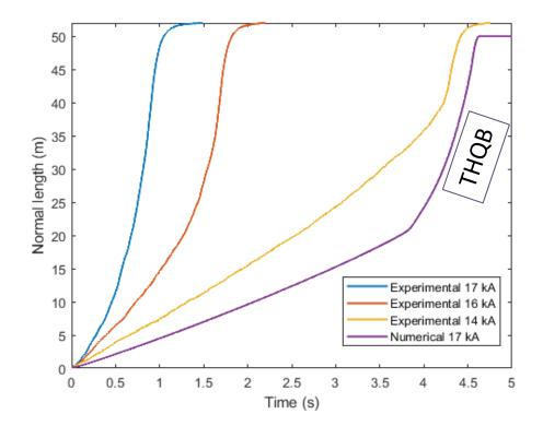
After normal quench initiation  $\rightarrow$  second quench propagation acceleration  $\rightarrow$  **Thermal Hydraulic Quenchback** phenomenon: pre-warming of the conductor by friction forces due to He flow
