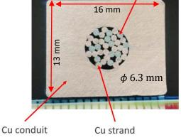
Quench propagation velocity tests with new conductor at CEA-Saclay, France
