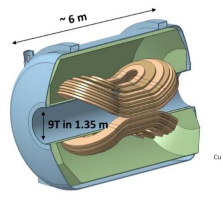
New conductor: CICC with Cu profile NbTi strand R&D Risk mitigation → **Quench propagation velocity** tests with new conductor using a dedicated solenoid magnet: **MA**dmax **C**oil for **Q**uench **U**nderstanding
