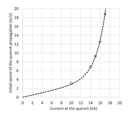
Quench propagation speed ~10 m/s; detection < 1 s (within specifications very successful results!)
