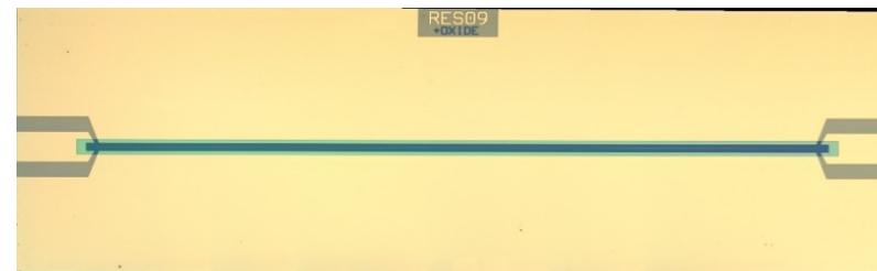
Resonator paramp. ~20dB gain at frequencies up to 18GHz.
