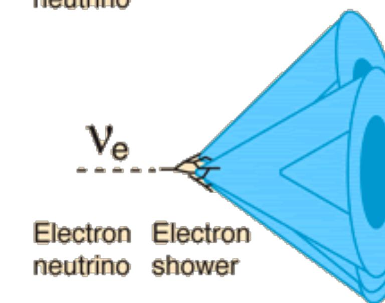
The Cerenkov radiation from the electron shower produced by an electron neutrino event produces multiple cones and therefore a diffuse ring in the detector array.
