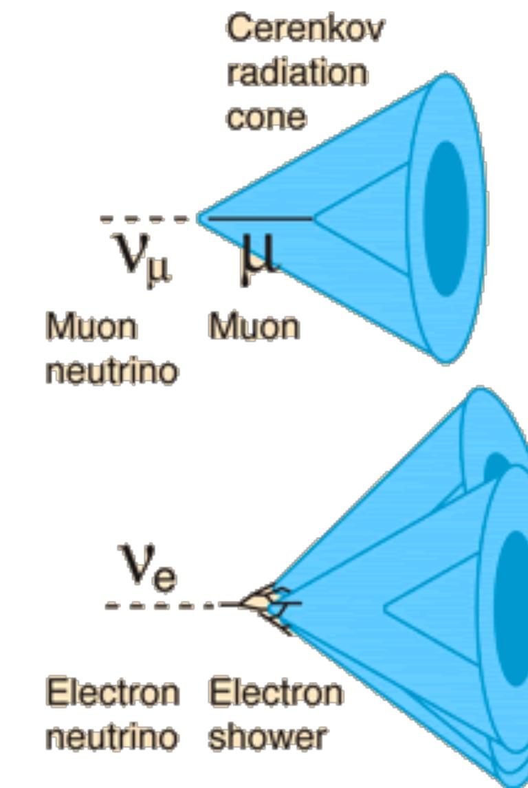
The Cerenkov radiation from a muon produced by a muon neutrino event yields a well defined circular ring in the photomultiplier detector bank.
