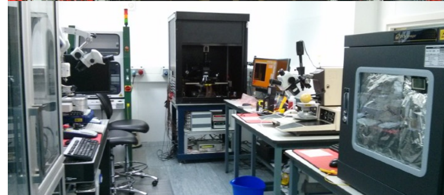
Example: Clean room used for sensor testing for the ATLAS upgrade programme
