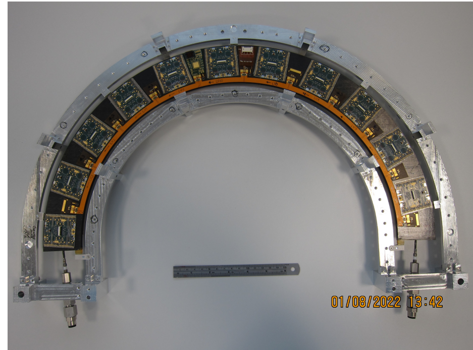
A Pixel half-ring fully loaded with working demonstrator (RD53A) modules, now undergoing electrical system testing.
