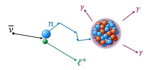
Gadolinium is used to capture neutrons ejected by antineutrino interactions
