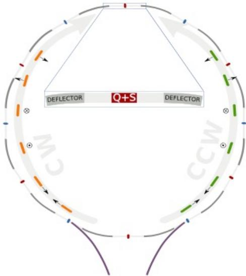
UK proposing to build E-field electrodes: stability & alignment of which limit the EDM sensitivity
