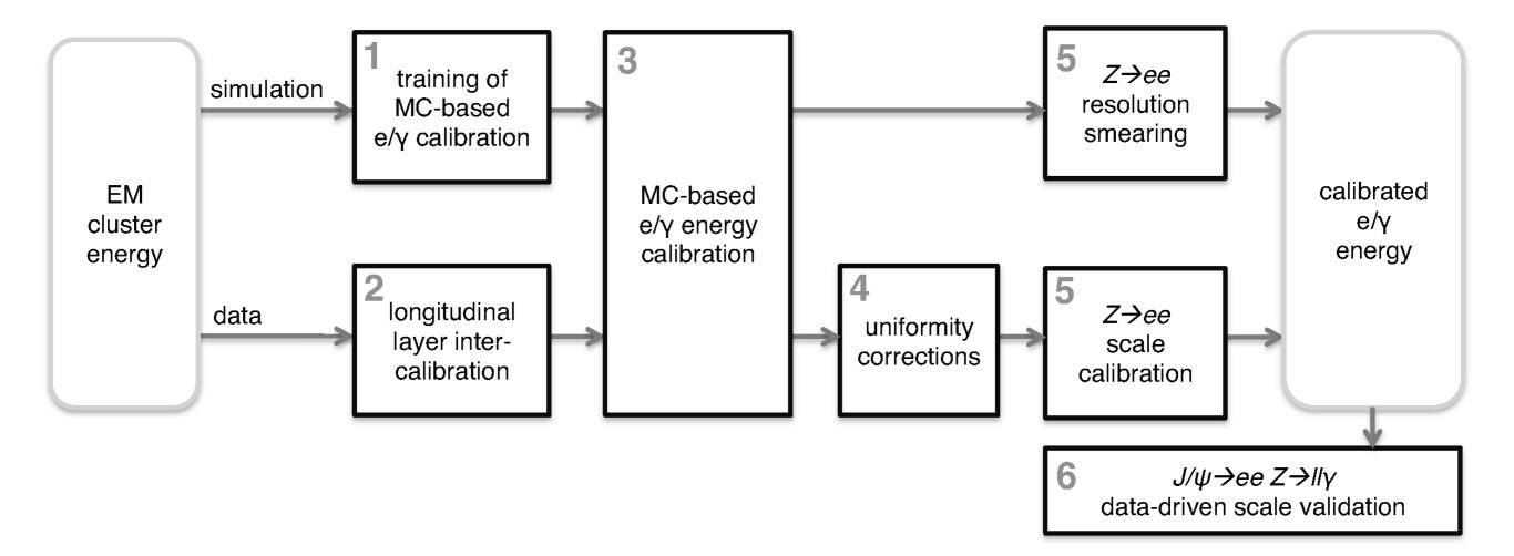
The different steps performed in the procedure to calibrate the energy response of electrons and photons from the energy of a cluster of cells in the EM calorimeter are the following:
