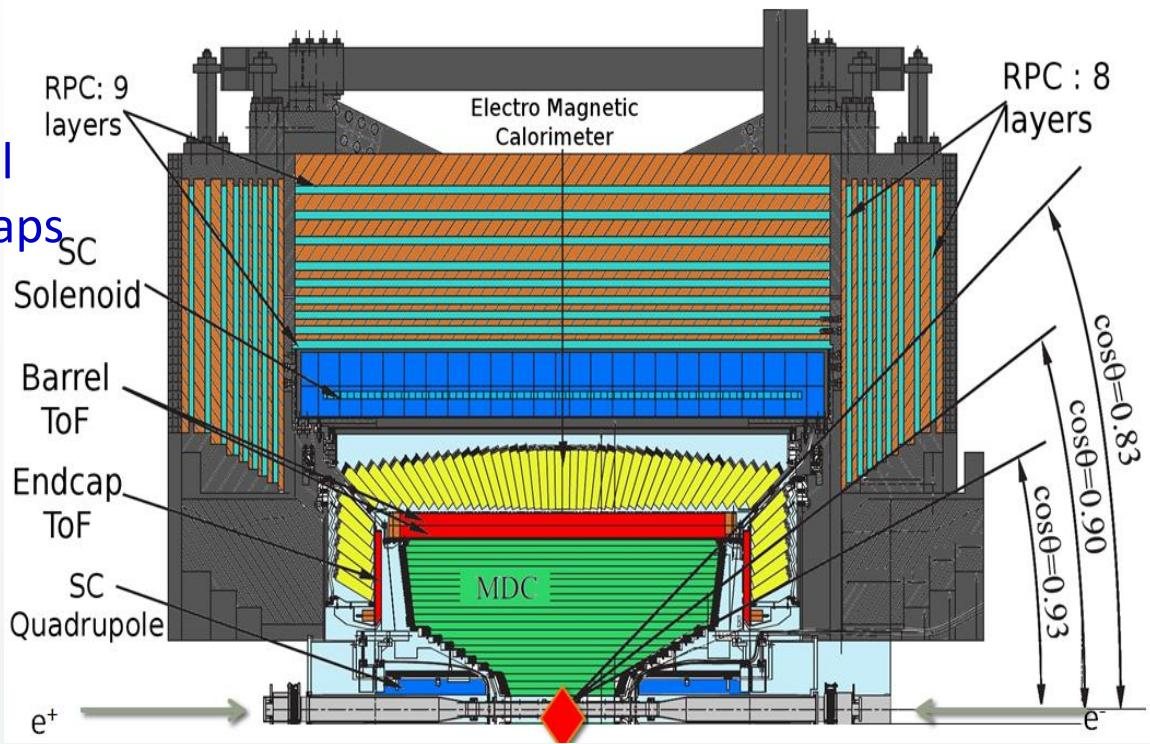
Total weight 730ton, ~40,000 readout channels
