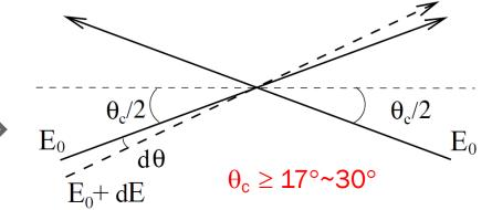
Existing monochromatization scheme for head-on collisions will reduce luminosity significantly New scheme: Provide the beams with an angular dispersion such that a beam particle arrives to the IP with a horizontal angle that depends on its energy.
