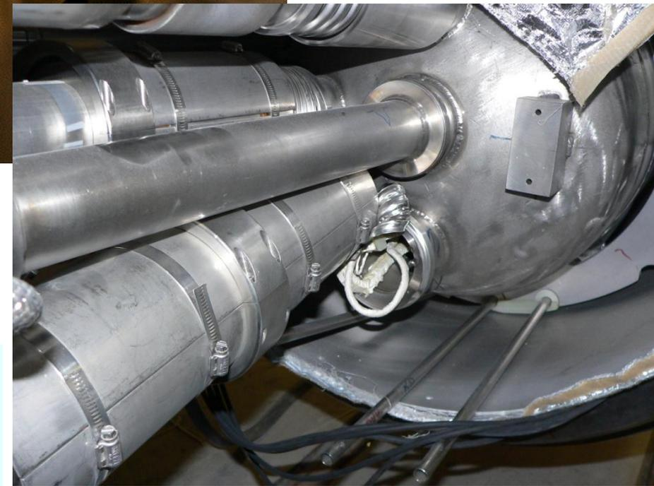
On Tuesday March 27 2007 there was a serious failure in a high-pressure test at CERN of a Fermilab-built “inner-triplet” series of three quadrupole magnets
