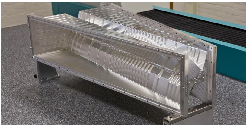
RF Foil, 150-250 \mu m thick, separates primary and secondary vacuum volumes
