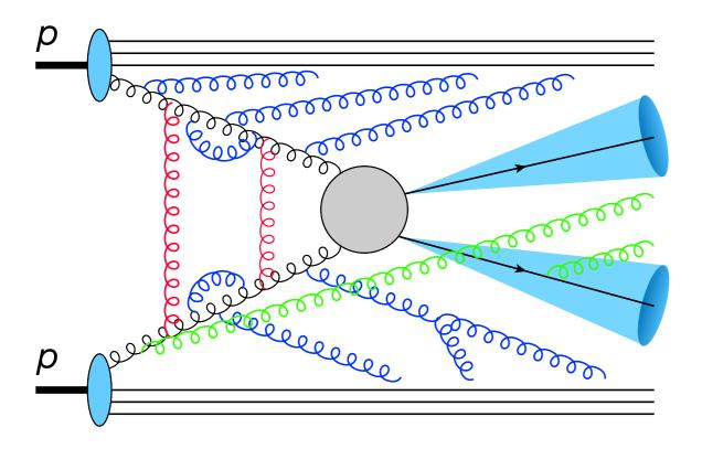
*red*: Coulomb gluons *blue*: gluons emitted along beams *green*: soft gluons between jets Loss of color coherence from initialstate Coulomb interactions
