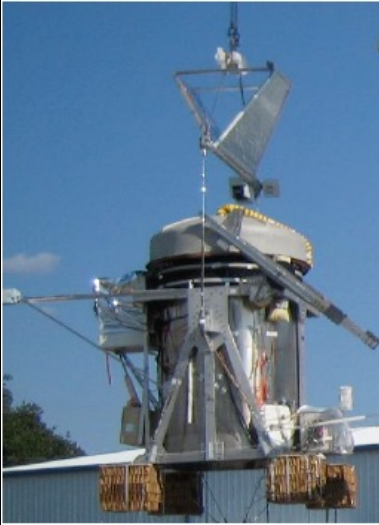
FIG. 5.— Photograph of the ARCADE 2 instrument just prior to 2006 flight. The instrument core is contained within the large (1.5 m diameter, 2.4 m tall) bucket dewar. The lid is shown closed
