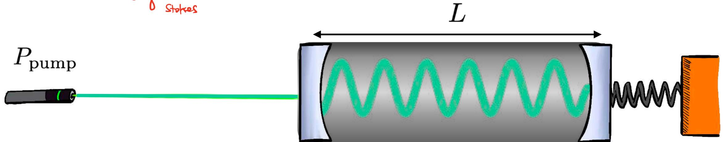
$$\omega_{\text{mec}} = n \frac{\pi}{L} c_s, \quad n \subset \mathbb{Z}$$
