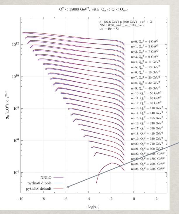
• Doubly-differential reduced cross section  $\sigma_R(x_B,Q^2) = F_2(x_B,Q^2) + \mathcal{O}(\alpha_s)$
