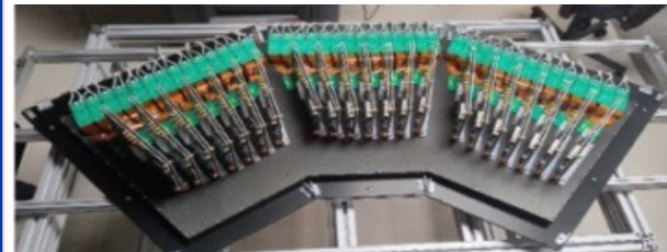
Full size prototype DTOF \sigma_t < 28 ps (cosmic ray test)
