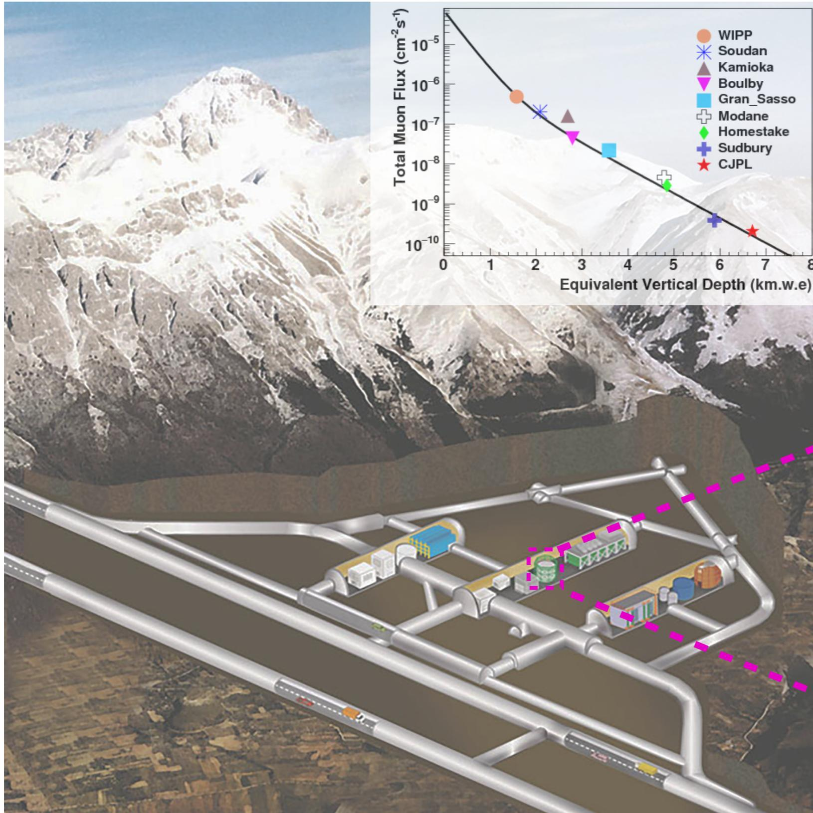
The INFN Laboratori Nazionali del Gran Sasso (LNGS) located under 1400 m of rock, shielding the laboratories from cosmic rays.
