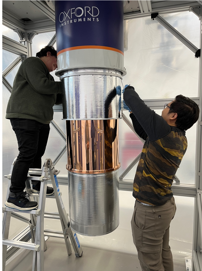
Nick Du and Claude Mostyn fitting intermediate thermal shields. Magnet is at the bottom
