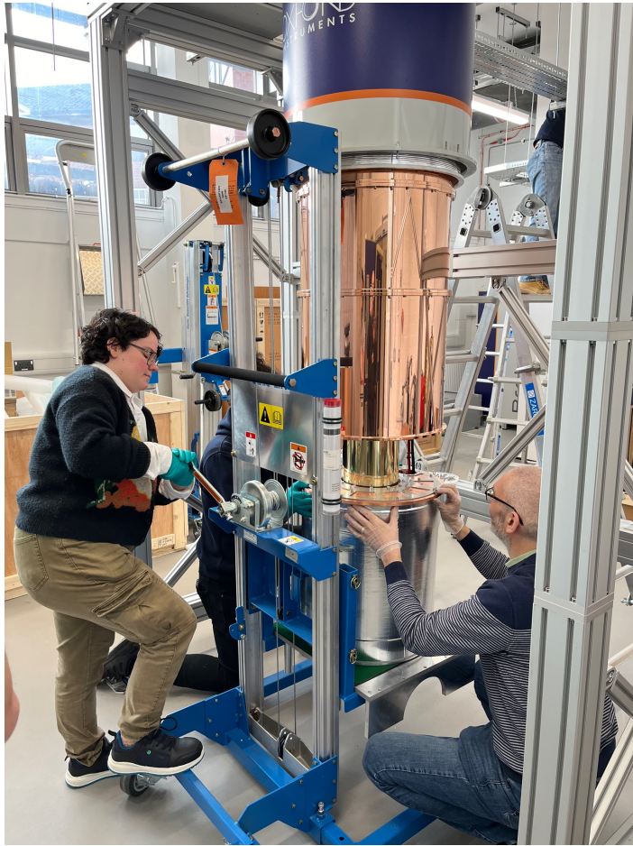
Claude Mostyn and Paul Smith (Sheffield) Jack magnet up to enclose 19cm diameter experimental payload space
