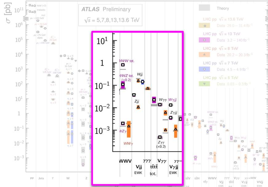
Measurement of the cross section of triboson production processes:
