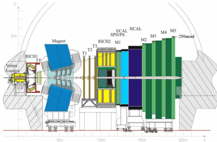
LHCb detector during Run1 and Run2
