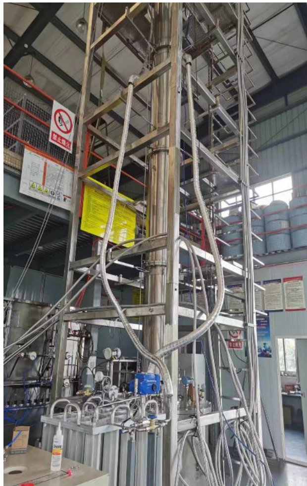
Kr distillation tower : 30 kg/hour. Target Kr concentration in Xe: 0.01 ppt
