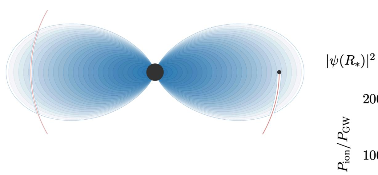
Perturber excites resonances in the cloud and it transitions from bound states to unbound states as the orbital frequency of the perturber hits the frequency of the energy difference between states
