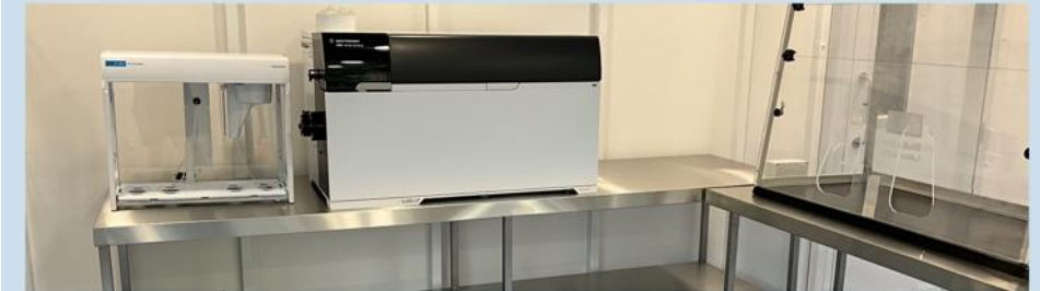
ICP-MS (Surface): Newly installed system for trace element analysis and isotopic ratio measurements.
