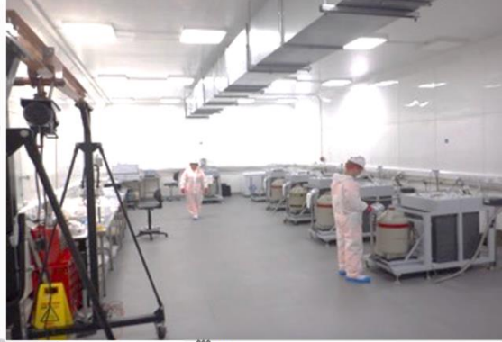
8 ULB Ge detector systems, 2 XIA alpha counters, 2 Rn emanation systems, ICPMS
