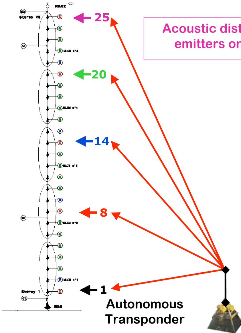
Acoustic distance measurement of hydrophones from fixed emitters on MILOM anchor + autonomous transponders
