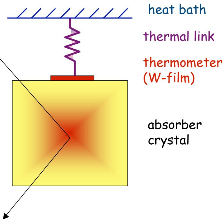
Particle interaction in absorber creates a temperature rise in thermometer which is proportional to energy deposition in absorber
