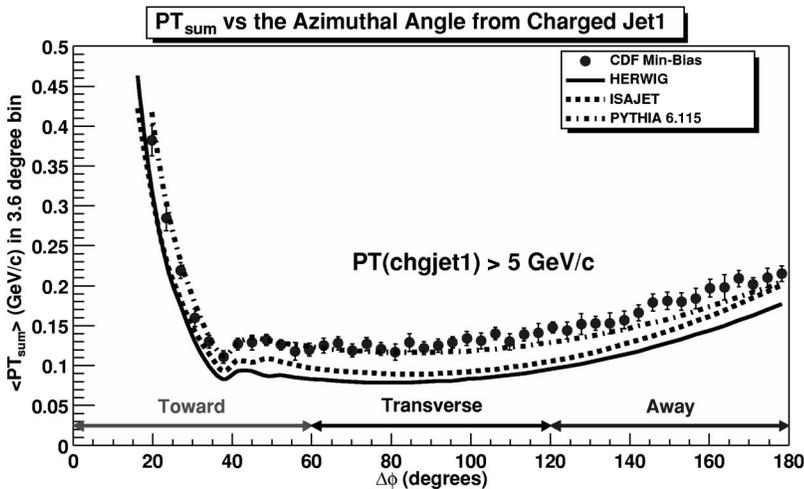
FIG. 18. Data from Fig. 16 on the average scalar  $p_T$  sum of charged particles ( $p_T > 0.5$  GeV/c,  $|\eta| < 1$ ) as a function of the relative azimuthal angle,  $\Delta\phi$ , between the particle and chgjet1 (leading charged jet) for  $P_{T1} > 5$  GeV/c compared to QCD Monte Carlo model predictions of HERWIG, ISAJET, and PYTHIA 6.115. The “toward,” “transverse,” and “away” regions defined in Fig. 14 are labeled.
