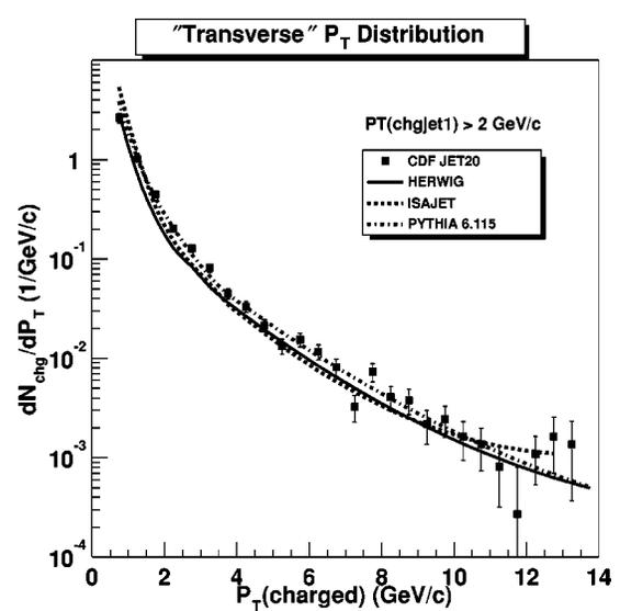
FIG. 41. Data from Fig. 37 on the transverse momentum distribution of charged particles ( $p_T > 0.5$  GeV/c,  $|\eta| < 1$ ) in the “transverse” region defined in Fig. 14 for  $P_{T1} > 30$  GeV/c compared to the QCD hard scattering Monte Carlo model predictions from predictions from HERWIG, ISAJET, and PYTHIA 6.115.
