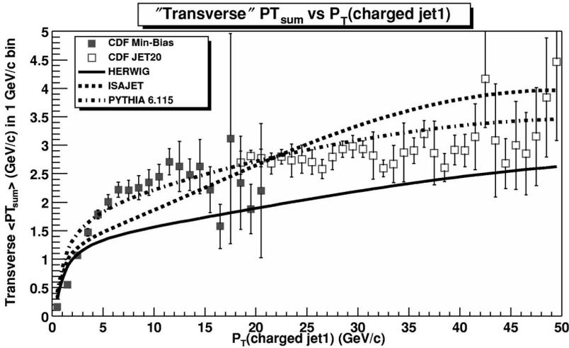
FIG. 29. Data from Fig. 22 on the average scalar  $p_T$  sum of charged particles ( $p_T > 0.5$  GeV/c,  $|\eta| < 1$ ) as a function of  $P_{T1}$  (leading charged jet) for the "transverse" region defined in Fig. 14 compared with the QCD Monte Carlo model predictions of HERWIG, ISAJET, and PYTHIA 6.115.
