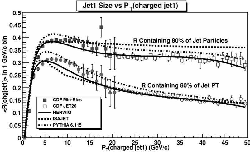
FIG. 6. The average radius in  $\eta$ - $\phi$  space containing 80% of the charged particles (and 80% of the charged *scalar*  $p_T$  sum) as a function of the transverse momentum of the leading charged jet compared with the QCD Monte Carlo model predictions of HERWIG, ISAJET, and PYTHIA 6.115. The solid (open) points are min-bias (JET20) data.
