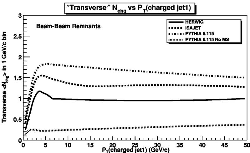
FIG. 36. QCD Monte Carlo model predictions from HERWIG, ISAJET, PYTHIA 6.115, and PYTHIA 6.115 with no multiple parton scattering (no MS) for the average number of charged particles ( $p_T > 0.5$  GeV/c,  $|\eta| < 1$ ) as a function of  $P_{T1}$  (leading charged jet) for the “transverse” region defined in Fig. 14 arising from the breakup of the beam particles (“beam-beam remnants”). For PYTHIA the “beam-beam remnants” include contributions from multiple parton scattering (see Fig. 2).
