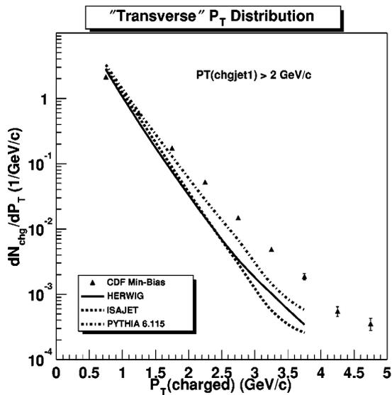
FIG. 39. Data from Fig. 37 on the transverse momentum distribution of charged particles ( $p_T > 0.5$  GeV/c,  $|\eta| < 1$ ) in the “transverse” region defined in Fig. 14 for  $P_{T1} > 2$  GeV/c compared to the QCD hard scattering Monte Carlo model predictions from predictions from HERWIG, ISAJET, and PYTHIA 6.115.
