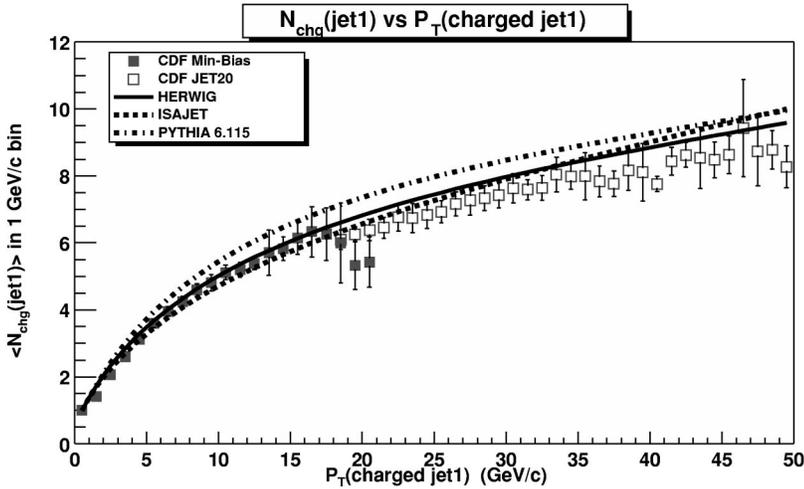
FIG. 4. The average number of charged particles ( $p_T > 0.5$  GeV/c,  $|\eta| < 1$ ) within the leading charged jet ( $R=0.7$ ) as a function of the transverse momentum of the leading charged jet compared with the QCD Monte Carlo models predictions of HERWIG, ISAJET, and PYTHIA 6.115. The solid (open) points are min-bias (JET20) data.
