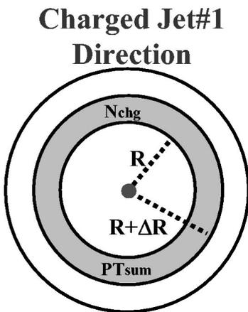
FIG. 7. Illustration of correlations in the radial distance  $R$  in  $\eta$ - $\phi$  space from the direction of the leading charged jet in the event,  $\text{chgjet1}$ . The average number of charged particles and the average *scalar*  $p_T$  sum of charged particles is plotted versus  $R$ , where  $R$  is the distance in  $\eta$ - $\phi$  space between the leading charged jet and a charged particle,  $R^2 = (\Delta\eta)^2 + (\Delta\phi)^2$ .
