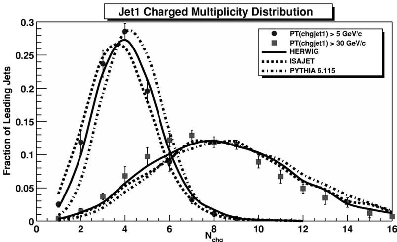
FIG. 5. Multiplicity distribution of charged particles ( $p_T > 0.5$  GeV/c,  $|\eta| < 1$ ) within chgjet1 (leading charged jet) for  $P_{T1} > 5$  and 30 GeV/c compared with the QCD Monte Carlo model predictions of HERWIG, ISAJET, and PYTHIA 6.115. This plot shows the percentage of events in which the leading charged jet ( $R=0.7$ ) contains  $N_{\text{chg}}$  charged particles. The  $P_{T1} > 5$  GeV/c points are min-bias data and the  $P_{T1} > 30$  GeV/c points are JET20 data.
