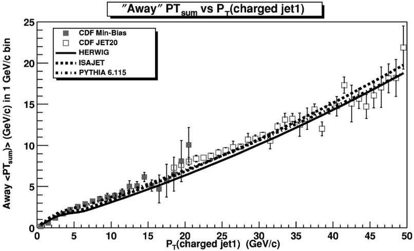
FIG. 26. Data from Fig. 22 on the average scalar  $p_T$  sum of charged particles ( $p_T > 0.5$  GeV/c,  $|\eta| < 1$ ) as a function of  $P_{T1}$  (leading charged jet) for the "away" region defined in Fig. 14 compared with the QCD Monte Carlo model predictions of HERWIG, ISAJET, and PYTHIA 6.115.
