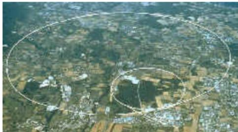
100 billion protons per bunch, 2800 bunches in each direction on **27 km length**, total beam energy of 300 Mega-Joules = 120 kg TNT, melts  $\approx 1$  ton of copper, collisions at 40 MHz  $\rightarrow$  1 Terabyte raw detector data per second, Higgs particle would be produced in 5 out of 1 billion collisions (J. Lykken: *Is particle physics ready for the LHC?*)
