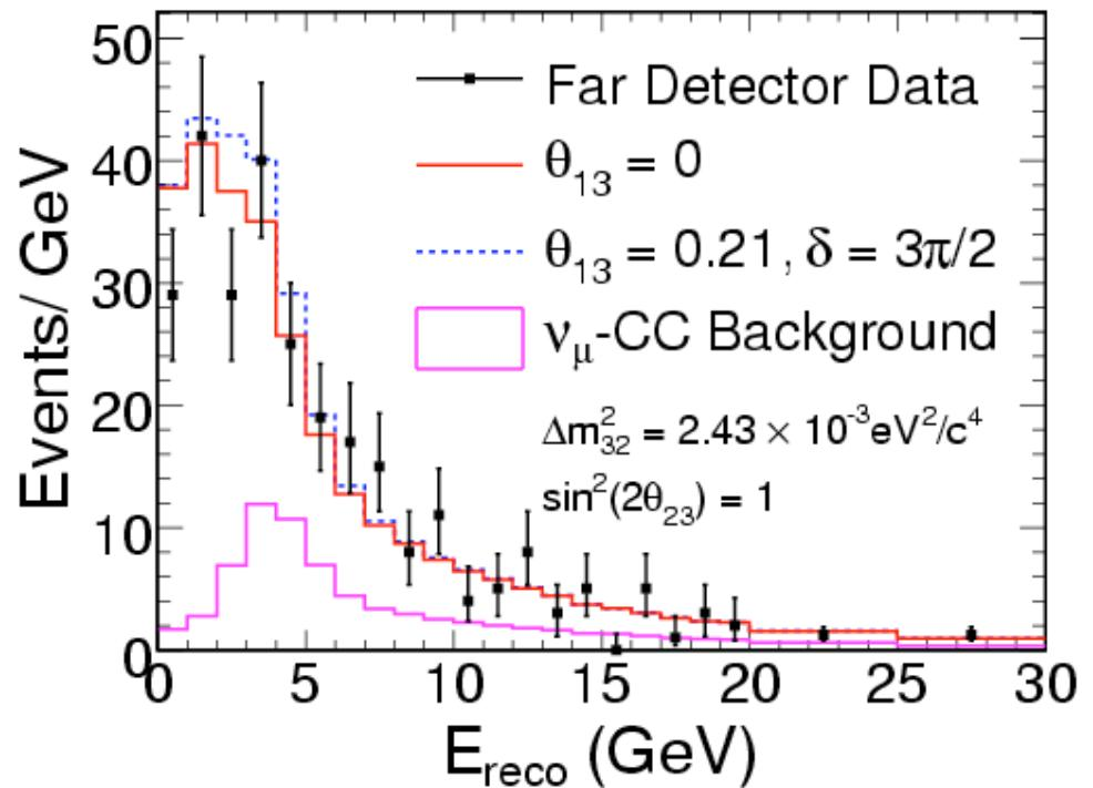
Simultaneous fit to CC and NC energy spectra yields the fraction of  $\nu_\mu$  that oscillate to  $\nu_s$ :
