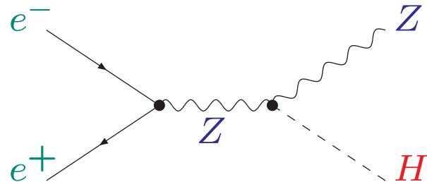
$$\sigma(e^+ e^- \rightarrow ZH) = \frac{G_\mu^2 M_Z^4}{96 \pi s} [v_e^2 + a_e^2] \beta \frac{\beta^2 + 12M_Z^2/s}{(1 - M_Z^2/s)^2}$$
