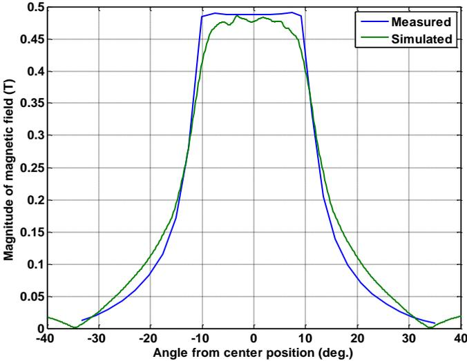
Simulated field from center of outside surface of rim, displaced 1 mm toward electromagnet
