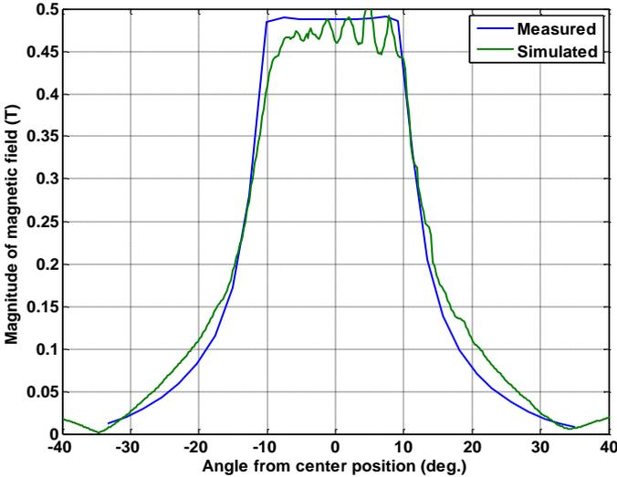
Simulated field from top of rim, displaced 1 mm away from electromagnet
