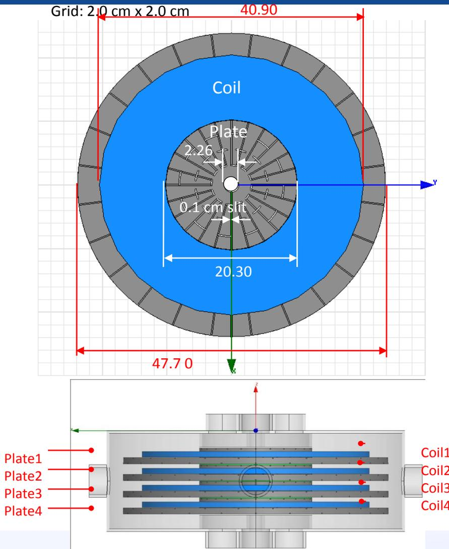
Note1: This geometry is our depiction of Wang's Flux Concentrator model where 4 Coils and 4 disks with a straight bore are modeled.
