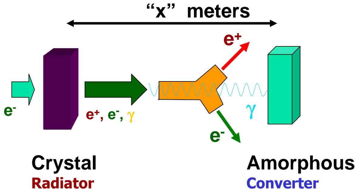
Only the photons are impinging on the converter: that limits the energy deposition in the amorphous target. The yield is less than if the particles coming from the crystal were also impinging on the amorphous target
