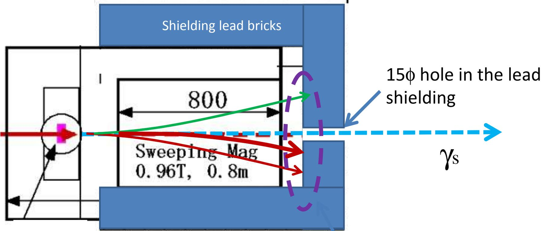
All charged particles are dumped here when the Sweeping magnet ON
