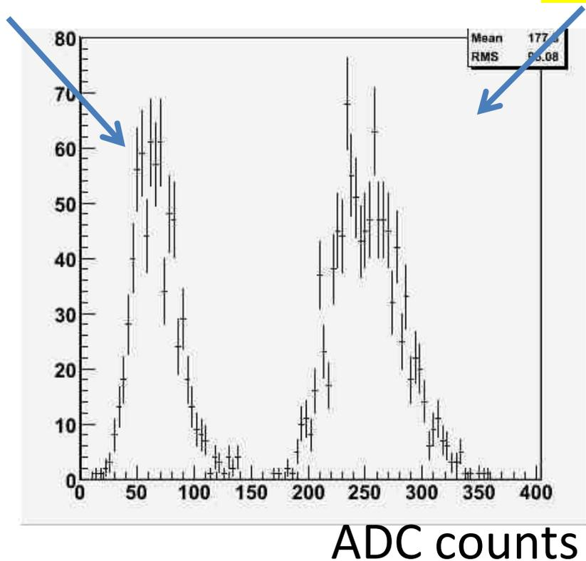
Signal is well separated from background even with NO converter
