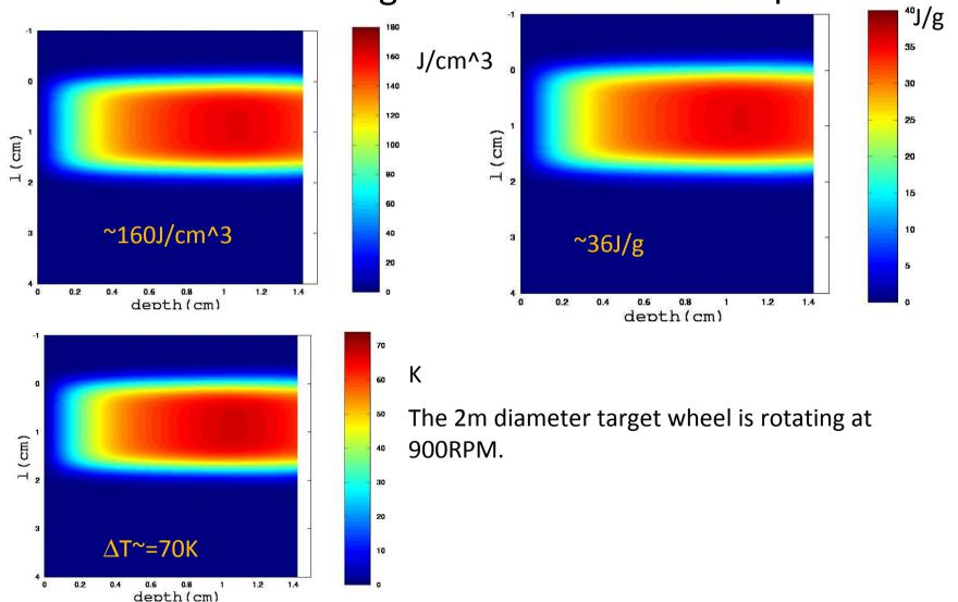
Energy density and estimated temperature change after 500 bunchs. RDR undulator, 250GeV drive, AMD Immersed 0.4X0 Ti target. 2e10 e+ assume captured
