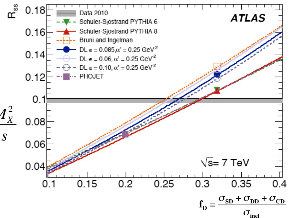
Figure 1: The ratio of the single-sided to inclusive event sample  $R_{ss}$  as a function of the fractional contribution of diffractive events to the inelastic cross-section  $f_D$ . The data value for  $R_{ss}$  is shown as the horizontal line with its systematic uncertainties (grey band). Also shown are predictions of several models as a function of an assumed value of  $f_D$ . The default  $f_D$  value (32.2% for all models but PHOJET which is 20.2%) is indicated by the markers.
