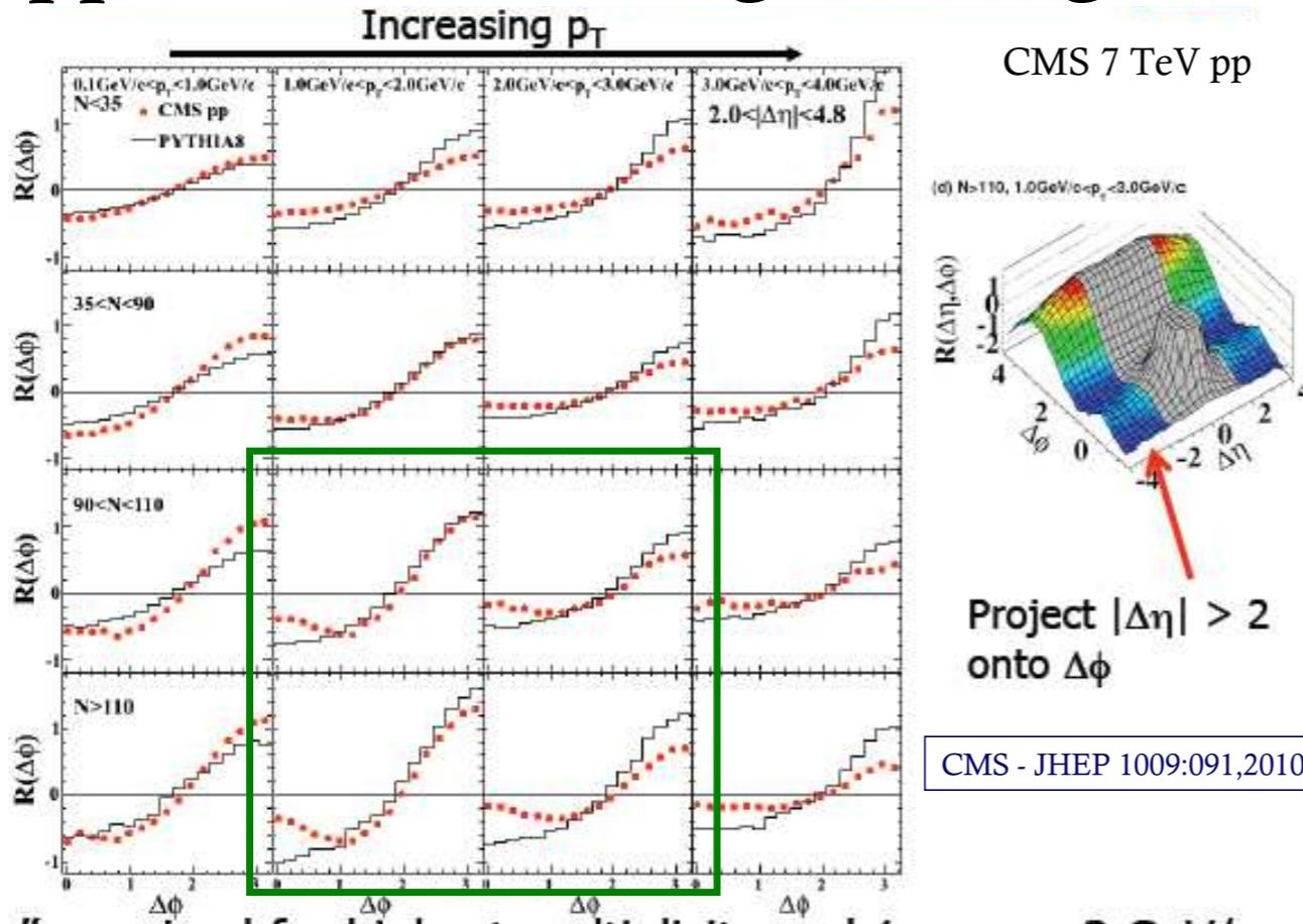
"Ridge" maximal for highest multiplicity and  $1 < p_T < 3 \text{ GeV}/c$
