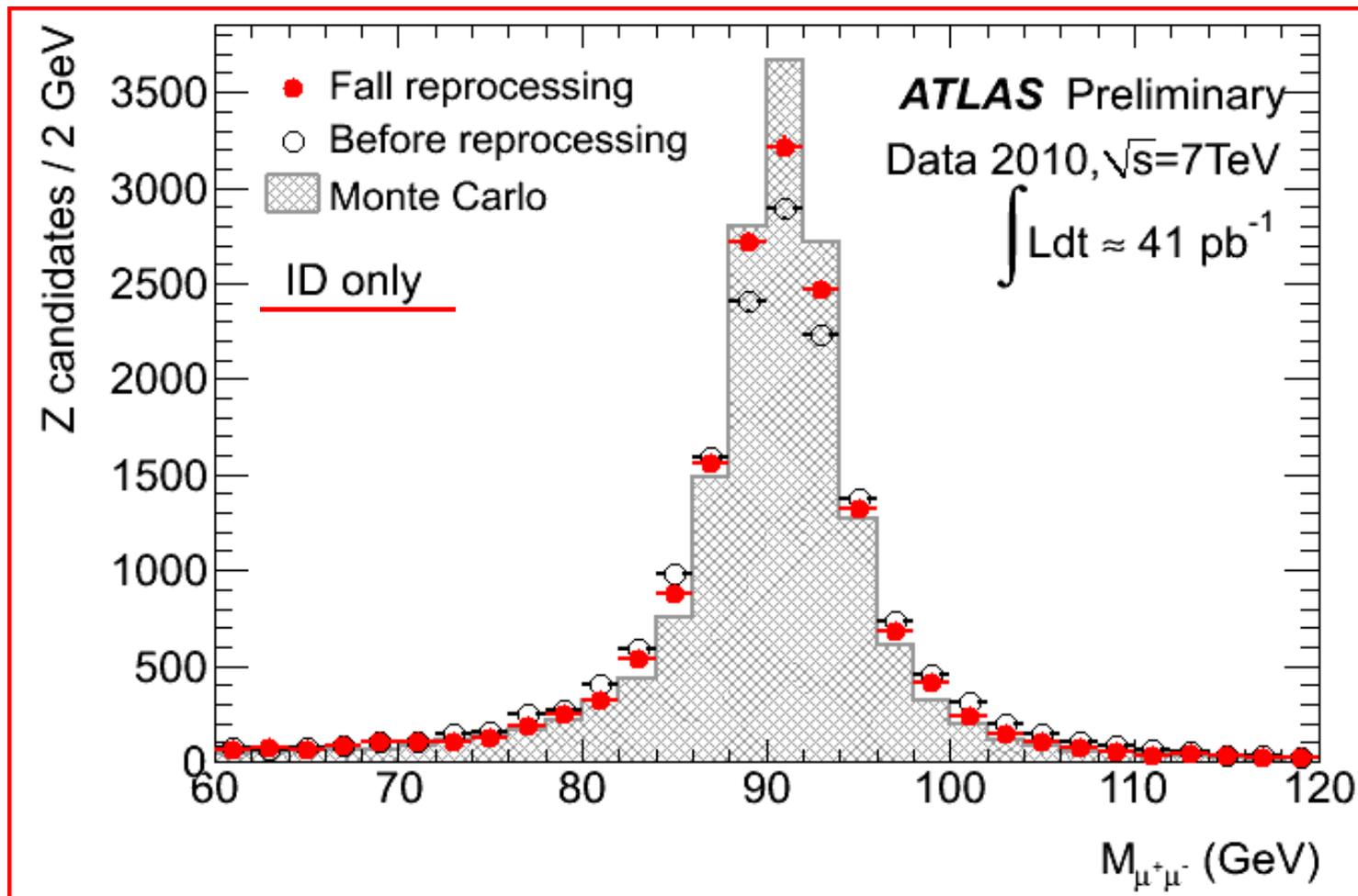
The effect of the new alignment on the Z mass reconstructed with ID tracks only. Before the processing is seen in the open circles and after seen in red.
