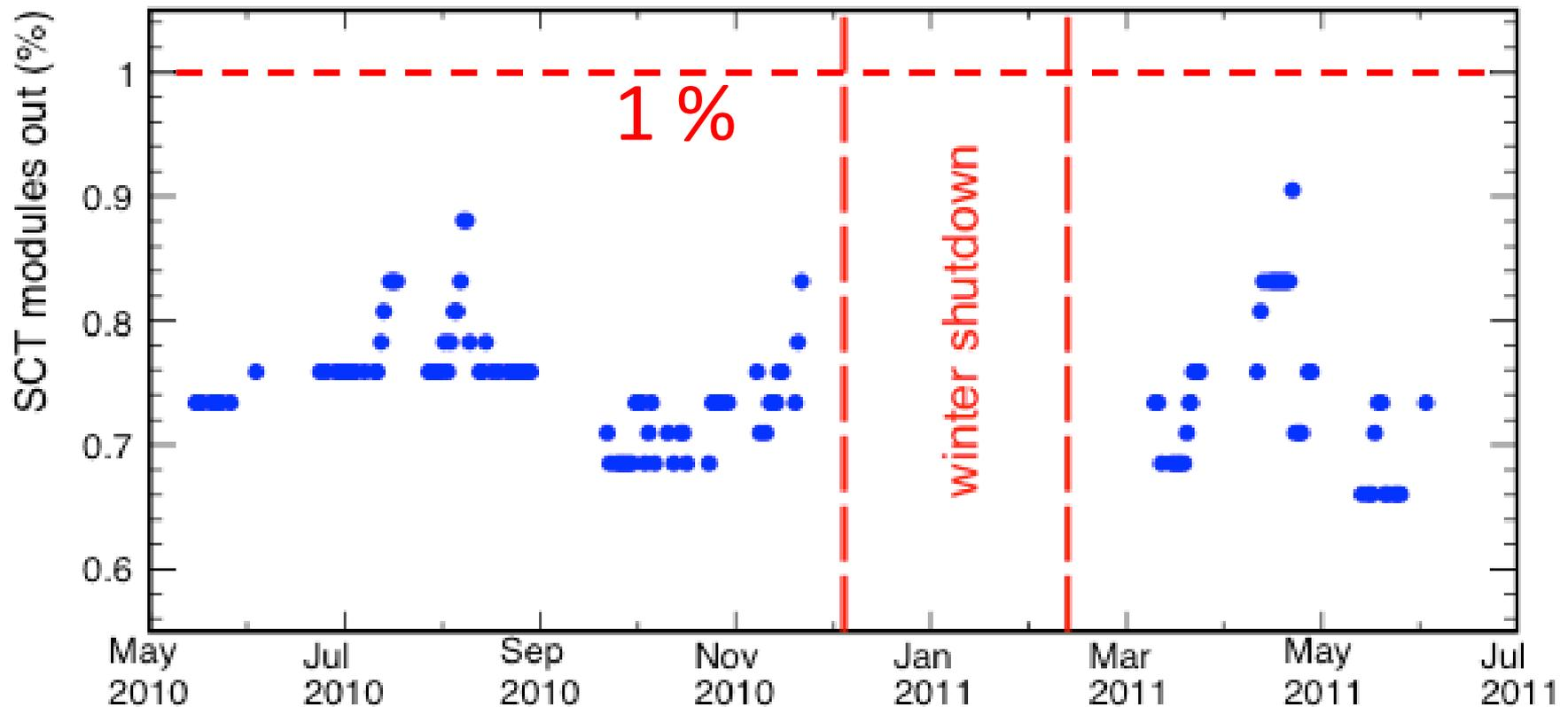
The number of SCT modules out of the physics configuration as a function of time during 2010 and 2011 up to June.
