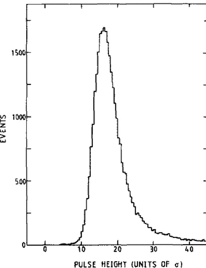
Fig. 5. Pulse height distribution for minimum ionizing particles.
