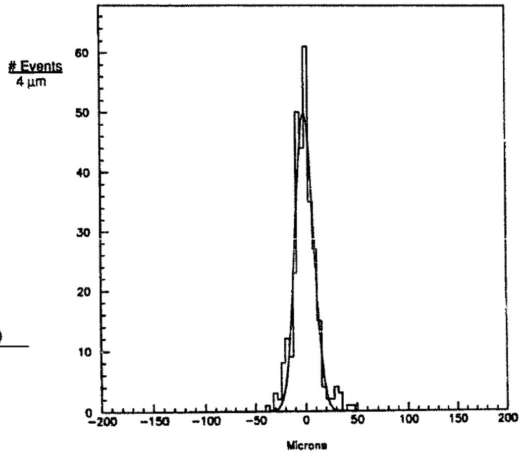
Fig. 8. Residues for the DELPHI half module.
