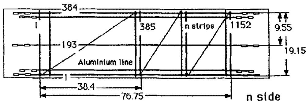
Fig. 6. The pattern of contacts between the two metal layers of a Closer layer detector (units are in mm).
