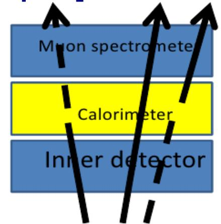
**Decaying signature:** energy deposition in calorimeter in events without collisions
