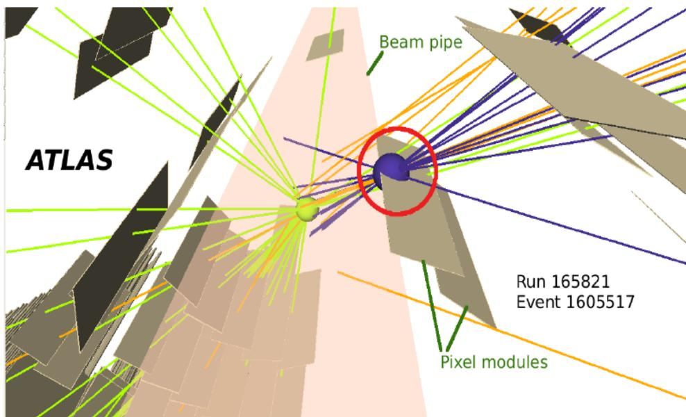
**Signature:** muon and secondary vertex from tracks, with large impact parameter, high track multiplicity, and high invariant mass
