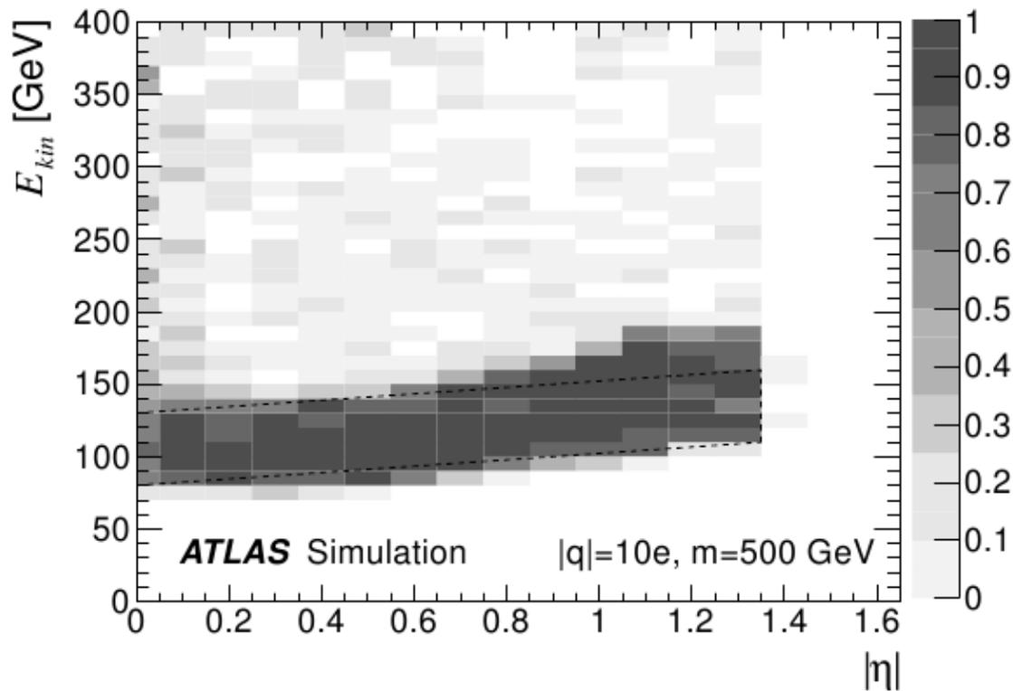
→ limits are set in well-defined kinematic ranges with high and flat signal selection efficiency (estimated from MC)
