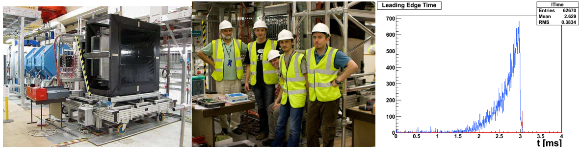
Figure 4 top: The EMR (test module of 6 planes) in the MICE hall in June 2011; the UNIGE team in front of the detector; the time structure of the MICE spill as recorded by EMR signals in beam.
