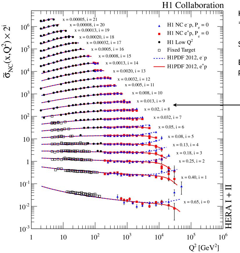
H1 precision I.5% for  $Q^2 < 500 \text{ GeV}^2$  $\Rightarrow$  factor 2 reduction in error wrt HERA-I
