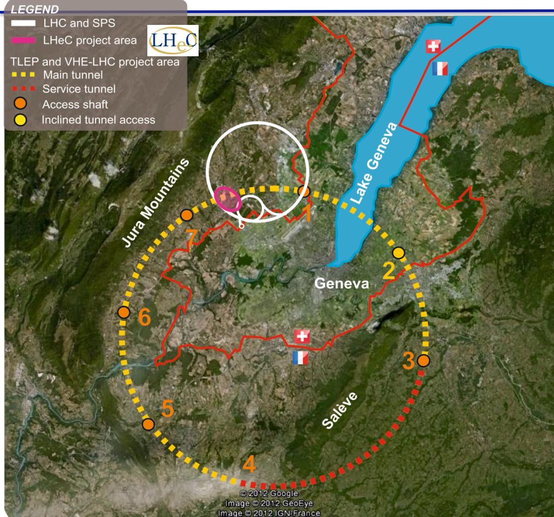
100 km with 20 T magnets provides 50 TeV per proton beam.
